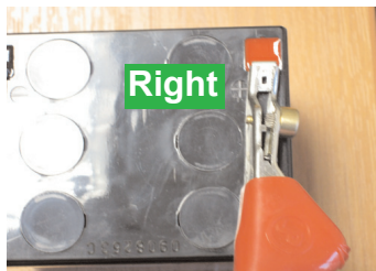
Grip clips tightly around tab terminals
